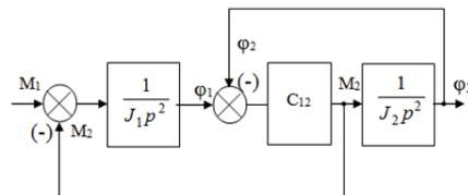
$$\begin{cases} \varphi_1 = \frac{M_1 - M_2}{J_1 p^2} \\ \varphi_2 = \frac{M_2}{J_2 p^2} \\ M_2 = C_{12}(\varphi_1 - \varphi_2) + C'_{12}(\omega_1 - \omega_2) \end{cases}$$
