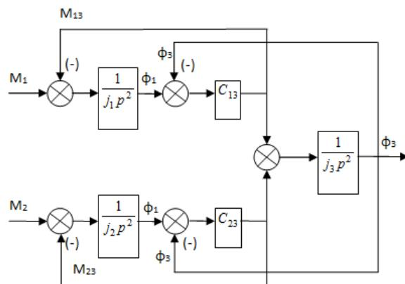
$$\left\{ \begin{array}{l} \varphi_1 = \frac{M_1 - M_{13}}{j_1 p^2}; \\ \varphi_2 = \frac{M_2 - M_{23}}{j_2 p^2}; \\ M_{13} = C_{13}(\varphi_1 - \varphi_3); \\ M_{13} = C_{23}(\varphi_2 - \varphi_3); \\ \varphi_3 = \frac{M_{13} + M_{23}}{j_3 p^2}; \end{array} \right.$$
